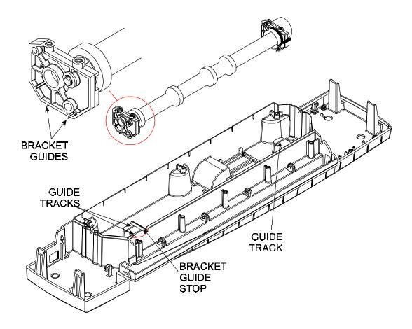
Figure 5-16. Installing Lower Roller Assembly.
